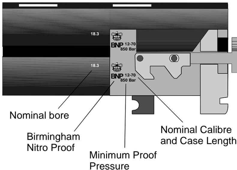
**Figure 3-1 – Typical proof marks on over-and-under barrels**
