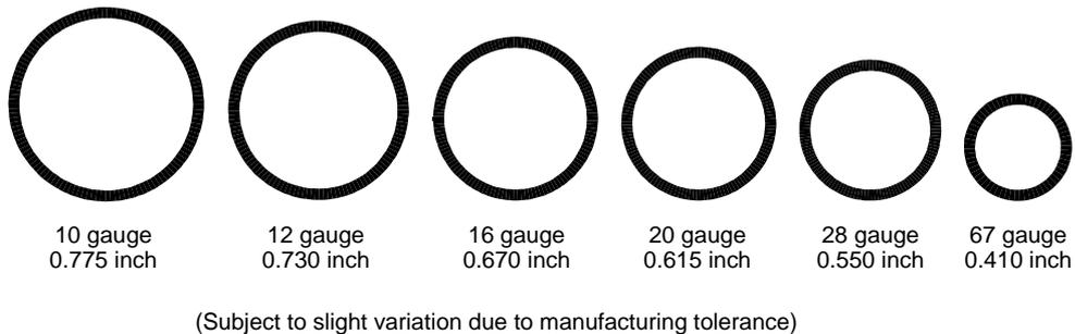
**Figure 1-5 – Bore Diameters**
