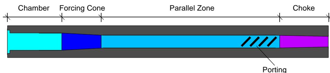
**Figure 1-9 – Barrel configuration**
