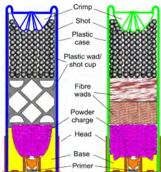
**Figure 2-1 – Cartridge construction**
