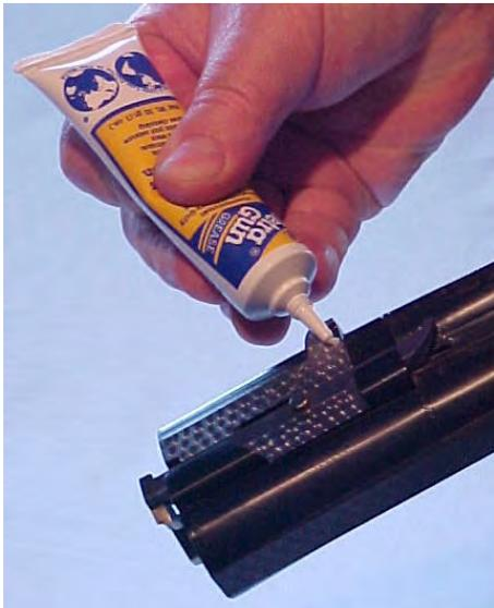
**Figure 1-16 – Grease the barrel hooks**
