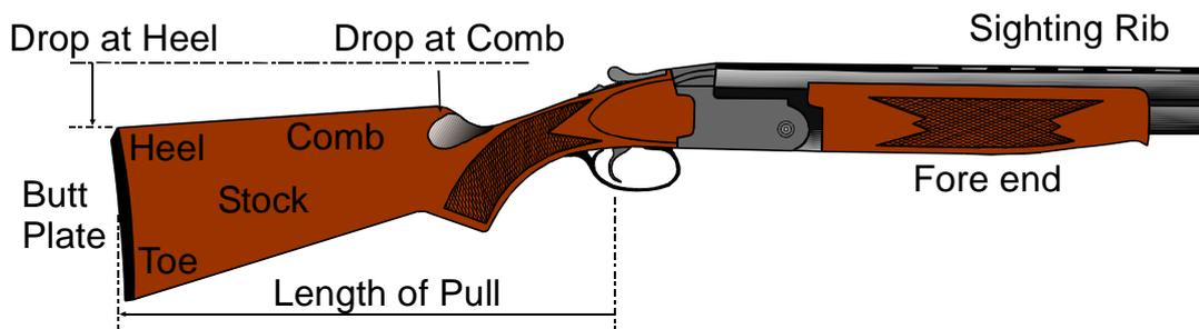
Figure 4-1 – The main dimensions of a stock
