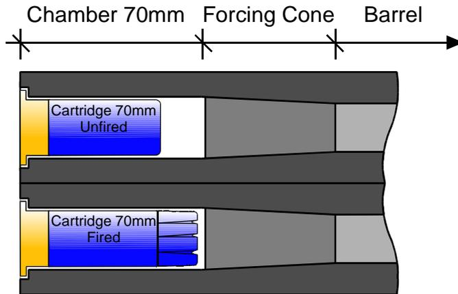
Figure 3-14 Cartridge/chamber length
