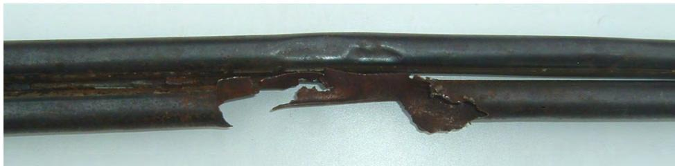
**Figure 3-13 – Barrel blocked by mud**
