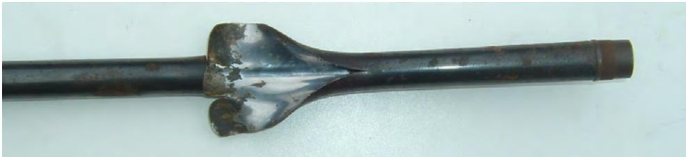
**Figure 3-12 – Barrel blocked by a wad**
