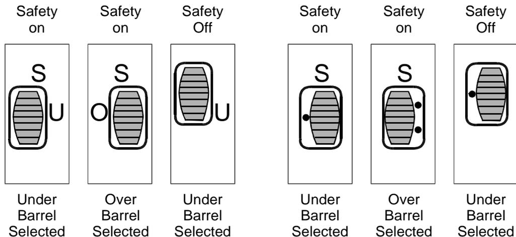
Figure 3-8 Safety catches with barrel selector markings
