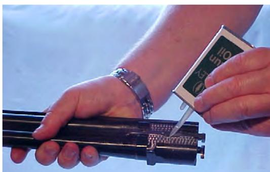
**Figure 1-13 – Oil the Ejectors**
