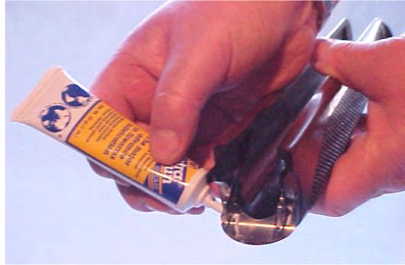
**Figure 1-15 – Grease bearing surfaces**
