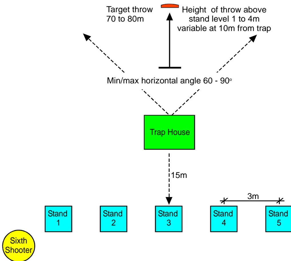
**Figure 7-3 – Automatic Ball Trap layout**
