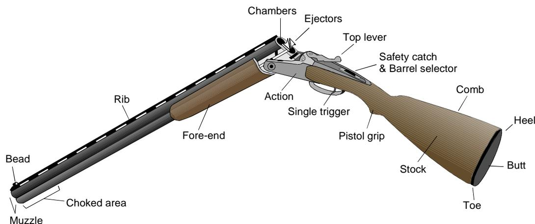
**Figure 1-8 Main components of a shotgun**
