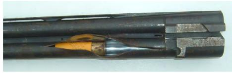
Figure 3-11 – A 20 bore cartridge in a 12 bore barrel
