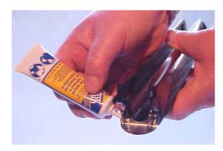
Figure 1-15 - Grease bearing surfaces
