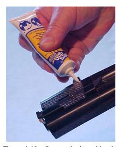
Figure 1-16 – Grease the barrel hooks
