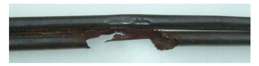
Figure 3-13 – Barrel blocked by mud
