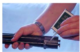
Figure 1-13 – Oil the Ejectors
