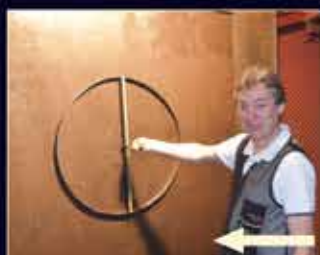
Finished pattern plate test - Confirming your finished comb height & cast are correct on your stock
