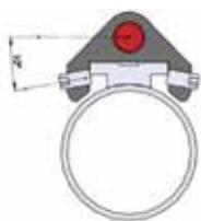
Sight positively locked to vent rib
