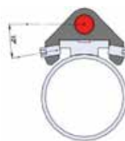
Sight positively locked to vent rib
