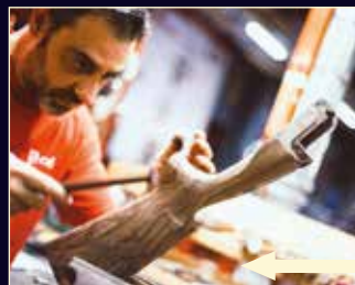
Alterations - Fine adjustments are made to the grip to suit your comfort & fit
