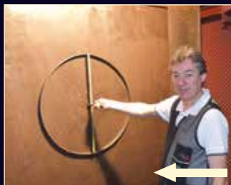
Finished pattern plate test - Confirming your finished comb height & cast are correct on your stock
